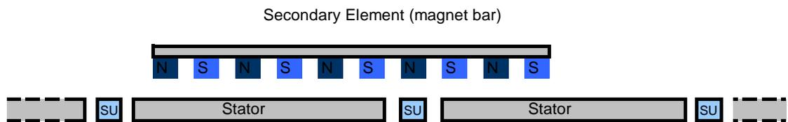
SU are usually mounted between each stators to determine the exact position of the Secondary Element by measuring the field across the Magnet Bar
