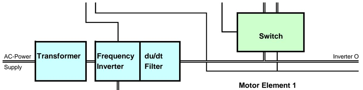
The Motor can be operated in an acceleration and brake mode. In the brake mode the energy fed back into the system has to be dissipated by means of a braking resistor.
