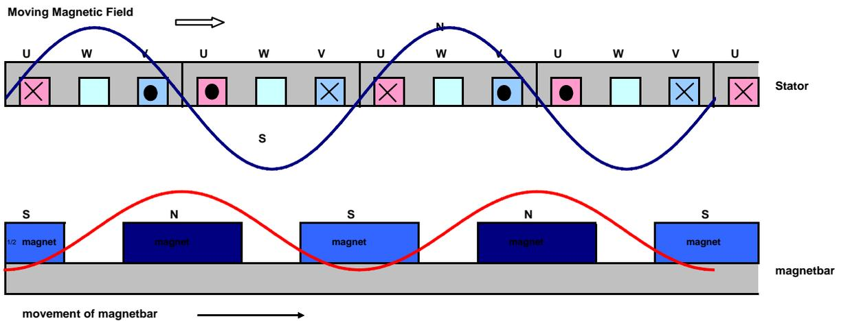
**Picture: Magnetic fields in the stator and secondary.**
