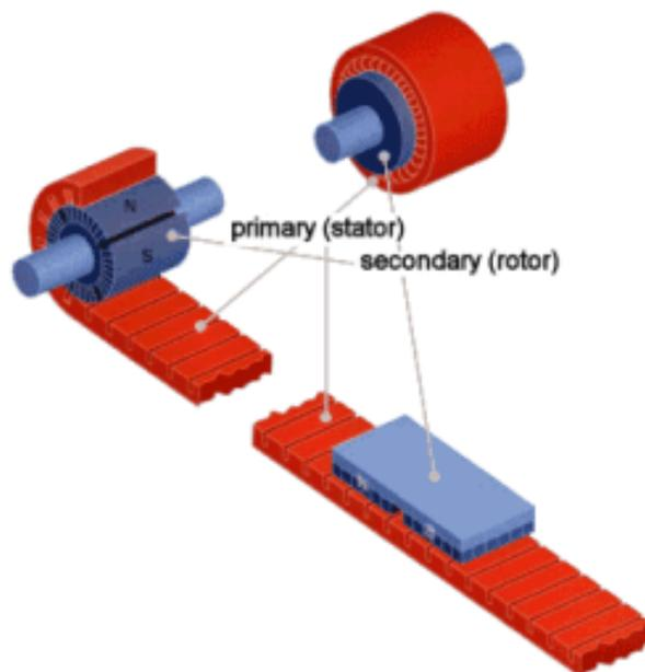
In a Synchronous Linear Motor (LSM) the secondary element consists of permanent magnets mounted alternately with N and S pole on a reactance core. The resulting magnetic field in a certain distance has a sinusoidal shape.
